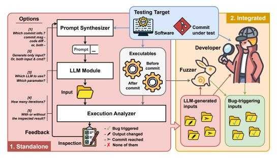
Fig. 1. CLEVEREST: Our zero-shot feedback-guided LLM-based regression test generation methodology.
